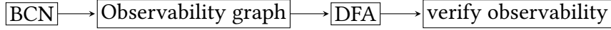
Figure 3.9: Sketch of using the notion of observability graph and finite automata to verify observability of BCNs.
