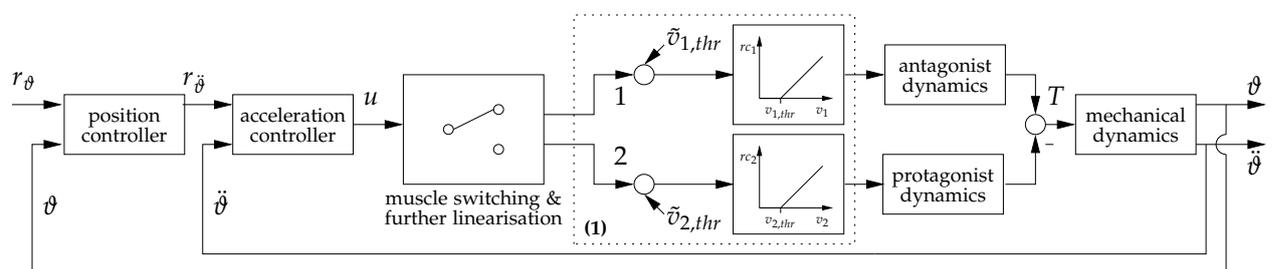
Figure 1: The acceleration control scheme applied to an antagonistic muscle pair.
