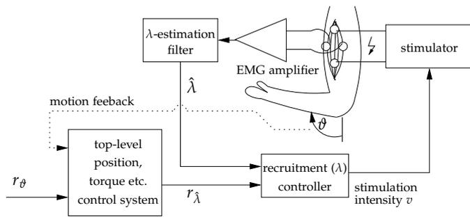
Figure 2: The  $\lambda$ -Control system exemplarily applied to the biceps
