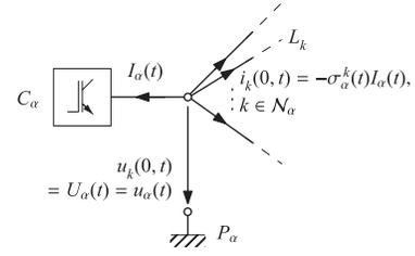
Fig. 5. Currents and voltages at the initial node  $P_\alpha$ ,  $\alpha \in \mathcal{P}_a$  of a tree-like network.
