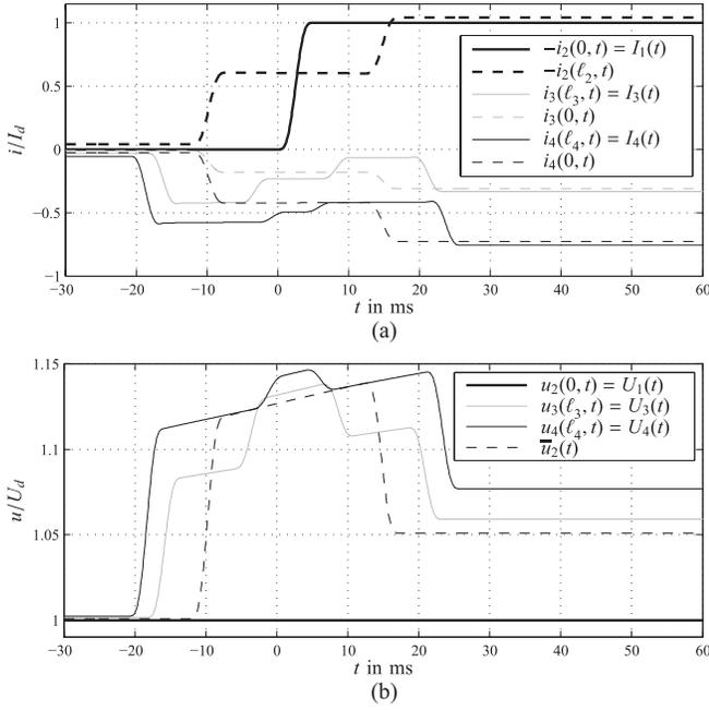
Fig. 10. Current and voltage trajectories for the three lines and converters during the transition between two states of rest for a change of the converter current  $I_1$  at converter  $C_1$  from the initial value  $\bar{y}_2^i = 0$  to  $\bar{y}_2^f = I_d$  via a polynomial trajectory on  $0 \leq t \leq \Delta t = 5$  ms. (a) Currents at the active nodes (solid line) and at  $P_2$  (dashed line). (b) Node voltages at the active nodes (solid line) and at  $P_2$  (dashed line).
