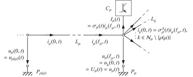
Fig. 6. Currents and voltages at one of the remaining nodes  $P_\mu$ ,  $\mu \in \mathcal{P}_a \setminus \{\alpha\}$  and the connected line  $L_\mu$  in a tree-like network.
