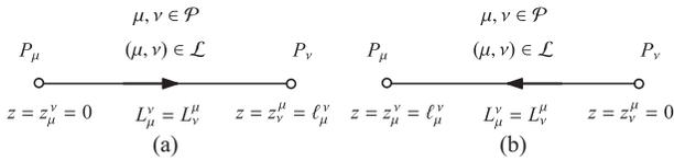
Fig. 2. Nodes and transmission lines in a general network. (a) Notation in case  $\mu < \nu$ . (b) Notation in case  $\mu > \nu$ .
