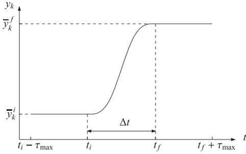
Fig. 7. Polynomial trajectory for one component  $y_k$  of the flat output  $y$  during the transition between two states of rest according to (16).
