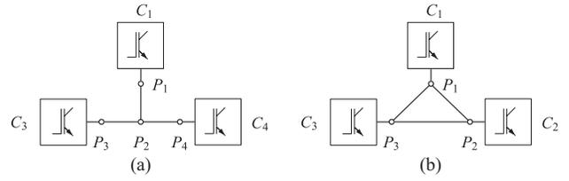
Fig. 8. Simple example networks with three converters. (a) Tree-like case. (b) General case with a line cycle.
