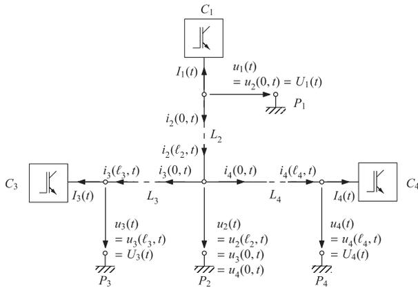
Fig. 9. Tree-like network with three converters and the notation for the case of  $P_1$  being chosen as initial node.
