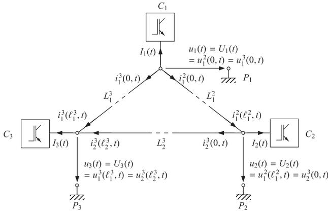
Fig. 11. General network involving three converters and a line cycle with currents and voltages at each node.
