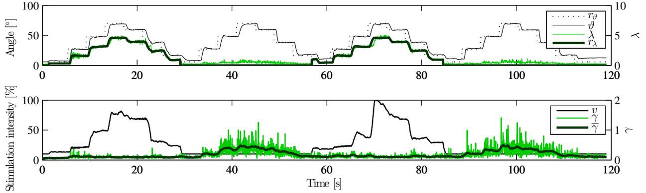
**Figure 2:** Results for a comparison of the FES-induced weight compensation to a pure voluntary muscle activation. The symbols are:  $r_{\vartheta}$  - target joint angle as displayed to the subject,  $\vartheta$  - joint angle,  $\lambda$  - muscular recruitment index,  $r_{\lambda}$  - desired recruitment level given to  $\lambda$ -control,  $v$  - stimulation intensity resulting from  $\lambda$ -control,  $\gamma, \bar{\gamma}$  - voluntary muscle activity.
