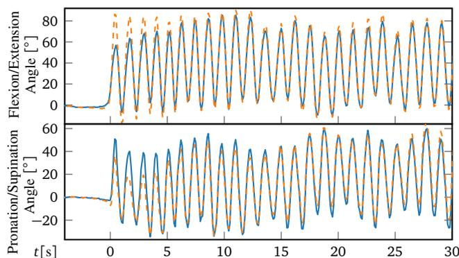
Fig. 5: Flexion/extension angle acquired by the optical reference measurement (—) and by using the IMU measurements together with the estimated axes (---). Correspondingly the pronation/supination angle is presented.
