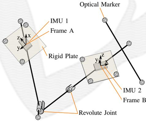
Fig. 1: Representation of the mechanical device resembling the human elbow joint. Shown are the two revolute joints, the two IMUs and the optical markers.
