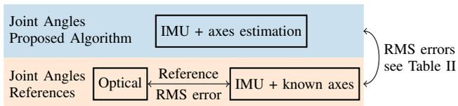
Fig. 2: The three sets of angles that are obtained for each experiment. The two reference angles are compared to the angles of the proposed algorithm as well as to each other.
