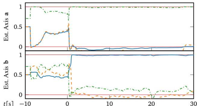
Fig. 4: The estimated axes of rotation of the mechanical device  $x$  (—),  $y$  (---) and  $z$  (-.-) and the expected constant axes values (—). In the second experiment the IMUs are placed on a layer of rubber foam to emulate skin motion.
