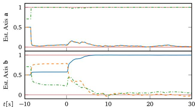
Fig. 3: The estimated axes of rotation of the mechanical device  $x$  (—),  $y$  (---) and  $z$  (-.-) and the expected constant axes values (—). The motion is started at 0s. In this experiment, the IMUs are rigidly attached to the mechanism.
