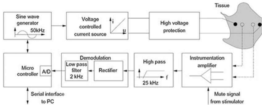
FIG. 1. Bioimpedance measurement system.
