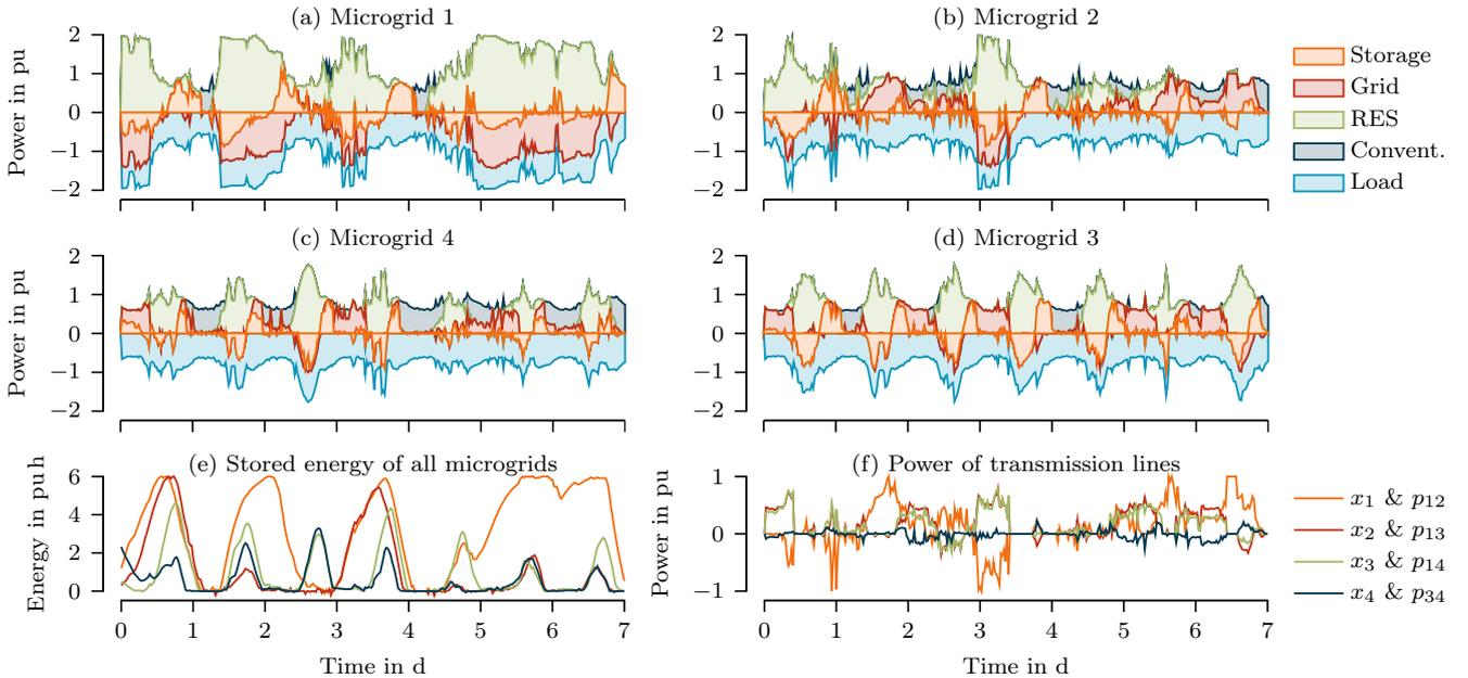
Fig. 6. Closed-loop simulation results obtained with distributed CC MPC approach.
