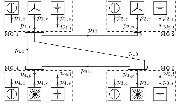
Fig. 1. Topology of four interconnected MGs from [6].
