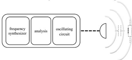
Fig. 3: Block diagram of a system that is able to detect changes in distance
