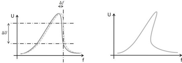
Fig. 6: Resonance curve of the new nonlinear LC-circuit; left: very steep flank; right: overhanging curve; Y-Axis: d.c. voltage
