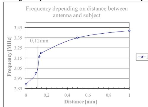
Fig. 10: Optimal distance between skin and antenna for obtaining maximum signal from sensor
