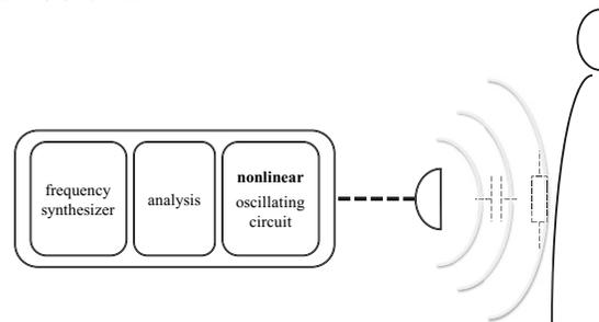
Fig. 5: Block diagram of the new system that uses a nonlinear oscillating circuit
