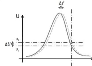
Fig. 4: Resonance curve of a linear LC-circuit. Y-Axis: a.c. voltage
