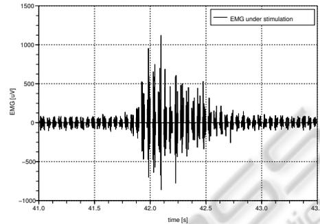
Figure 5: EMG recording of volitional muscle activity from the stimulated wrist extensor (pulse width  $100\mu s$ ,  $I=15\text{ mA}$ ).
