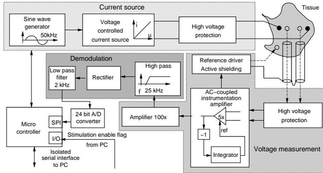
Fig. 1 Block diagram of measurement device.
