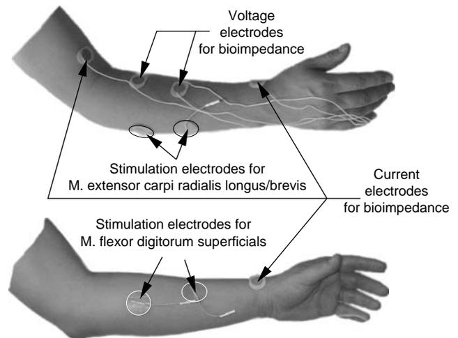
Fig. 3 Electrode positions.
