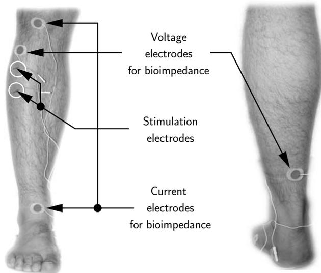
Fig. 5 Electrode positions for ankle-joint angle measurement.
