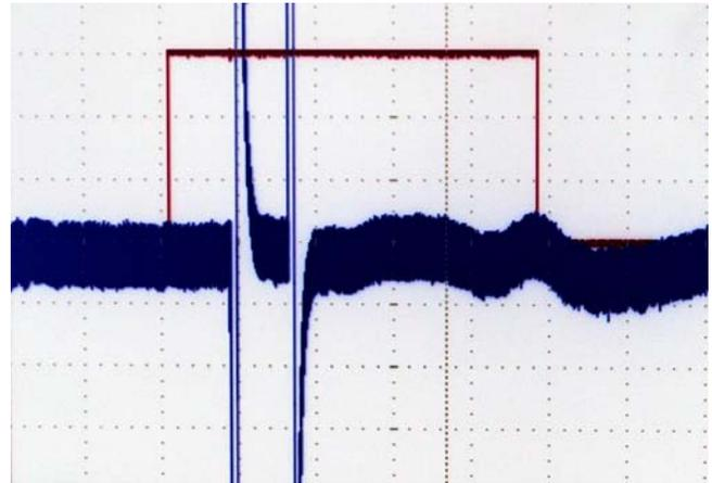
Fig. 2 Two stimulation impulses during bioimpedance measuring.
