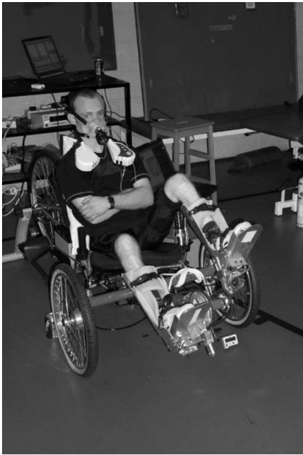
Fig. 1. Recumbent tricycle mounted on a trainer; subject connected to portable breath-by-breath gas exchange system.
