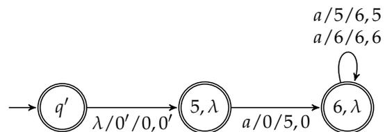
Figure 3.28: converted into DPDA with new stack bottom  $0'$
